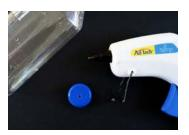
Step 2: Gently insert the hot tip of the glue gun into the center of the water bottle lid, melting a hole in it.
