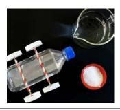
Step 6: Time to race! Take your car outside- this gets messy. Twist open the water bottle and pour 1 cup of vinegar into the water bottle. Add 1 tablespoon of baking soda and close cap. Shake and watch your car race off!
